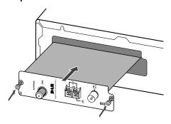
When the board meets the internal connector, apply a little more pressure so that the board plugs fully into the connector. Make sure the board's panel is flush with the T-4555's rear panel.
